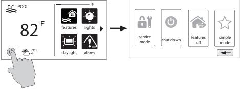
**Shut Down** - When Shut Down is selected, the OmniHub will turn off all pool equipment and report when it is safe to remove power. When this message is displayed, you can either power off the unit or restart the OmniHub by touching the large power button displayed on the left side of the screen.
